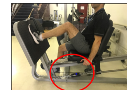
Fig 2. Load cell, attached to leg press.
